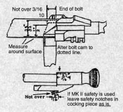
WHEN GRINDING NEW SAFETY NOTCH CHECK NO. 9 ABOVE. THESE MEASUREMENTS MAY VARY SLIGHTLY IN DIFFERENT ACTIONS.
