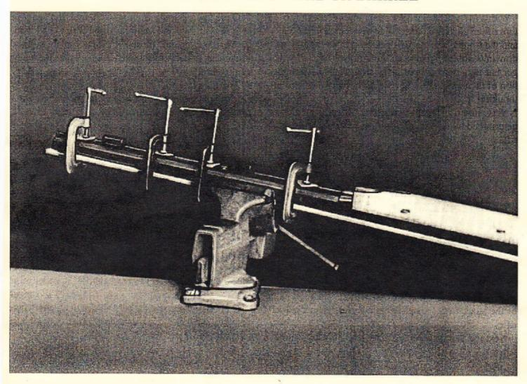
With all these operations complete and the rib screwed to the barrel, remount the barrel in the stock and check that you have clearance for the rib to pass the nose cap when the barrel is hinged down in the stock. If the rib contacts the nose cap, preventing the barrel from seating completely, remove a small amount of metal from the under rib to allow passage.
