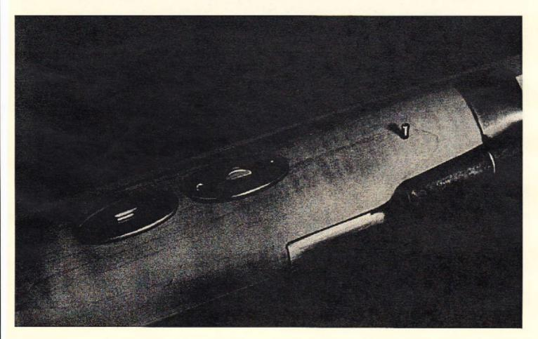
After you have made your initial inletting cuts, again place the escutchen on the stock and pass the key through it. Tap lightly and remove. You will now be able to see where the inlay has compressed the wood along the edge of the inletting, showing you where more wood needs to be removed. It is a good idea to scratch an arrow on the inlay so you can determine that you are putting it on the stock the same way each time you try the fit of the inletting.
