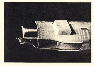
Use inletting black and fit this piece so that the groove for the ram rod lines up with the inner surface of the hole in the entry thimble. At the same time, maintain a good match on the vertical line of the nose cap where it meets with the stock.
