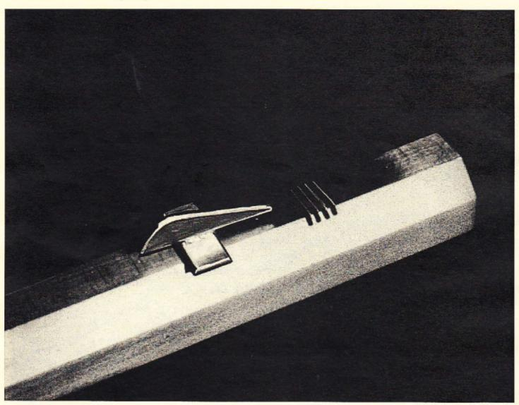
As of this writing rivisions are being made to add more "meat" to the top edge of the triggers (whee they come in contact with the sear) thereby allowing the builder to keep the correct alignment of trigger bar by taking metal off the top edge of triggers as he inlets the unit into stock. This goives our trigger unit capabilities of being used on other guns where regulating this height becomes essential.
