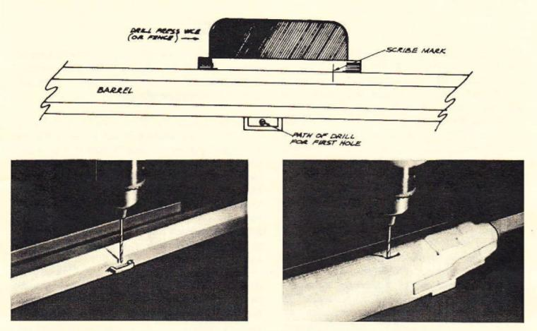
(The fence can be a piece of angle iron clamped to the drill press table with C-clamps, the drill press vise, or any other fixed surface which is fixed to the drill press table.)
